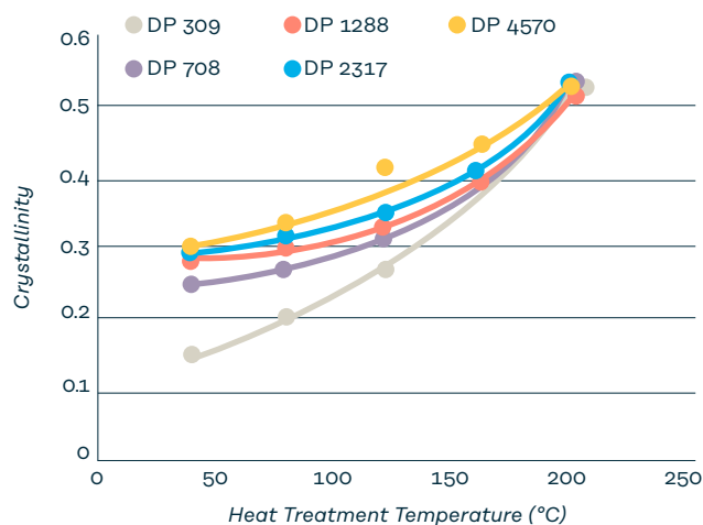
Figure 7. PVOH Film Heat Treatment Temperature (10 min) and Crystallinity
